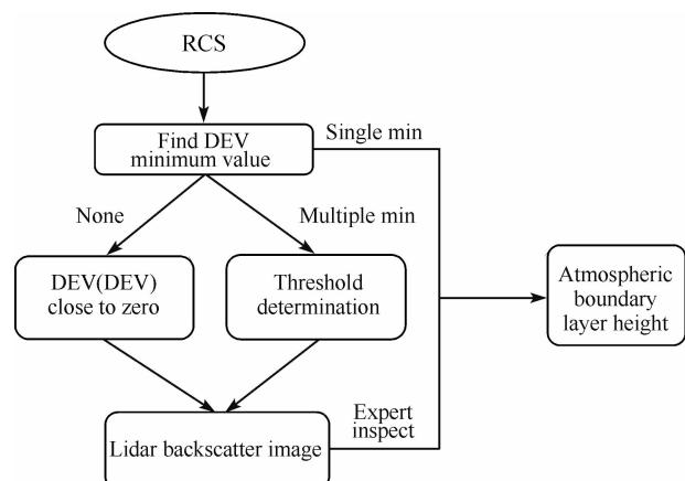
Fig.1 Flow chart of gradient method to detect the ABLH
