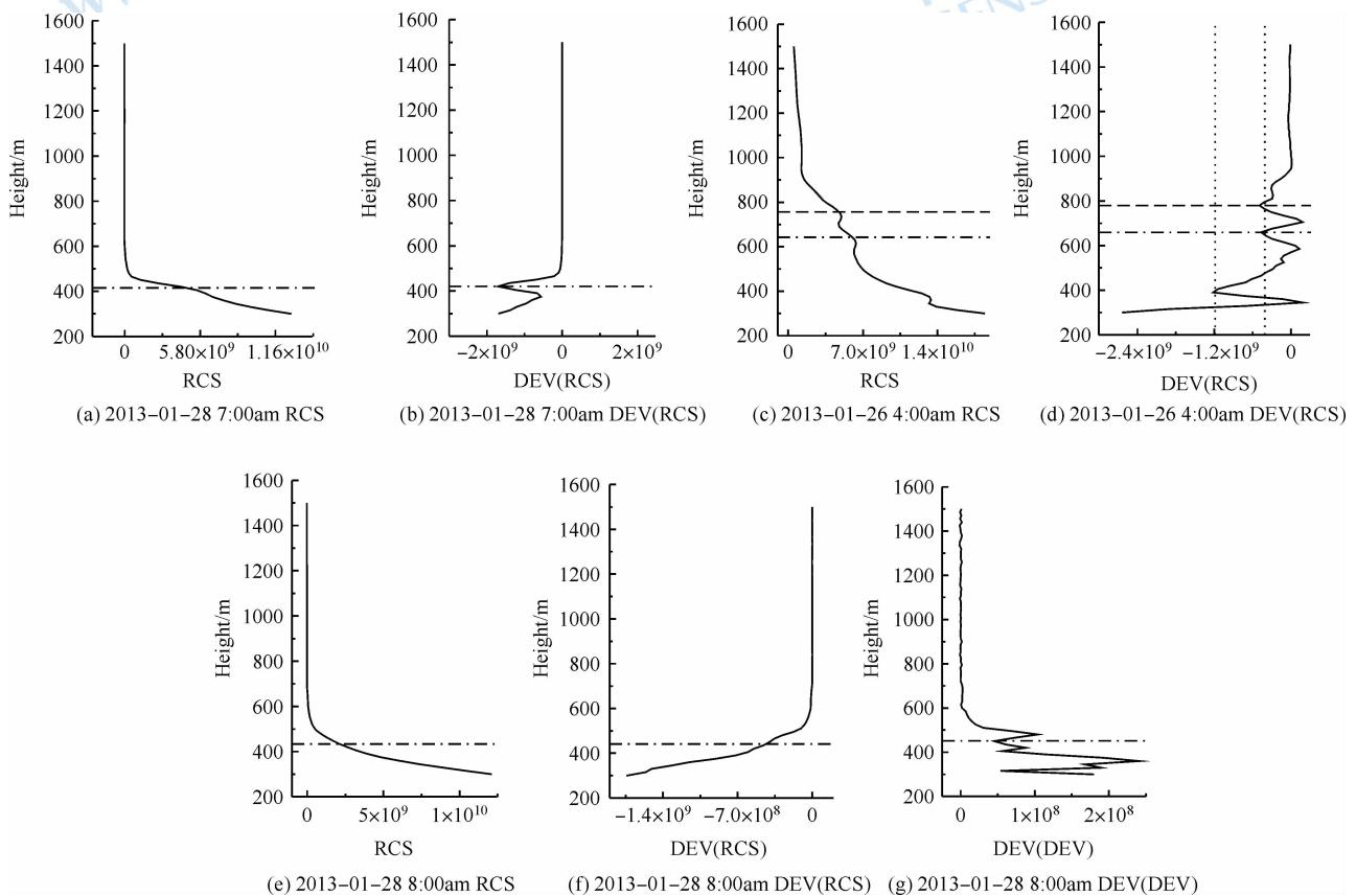
Fig.2 Interpretation of the gradient method to detect the ABLH
